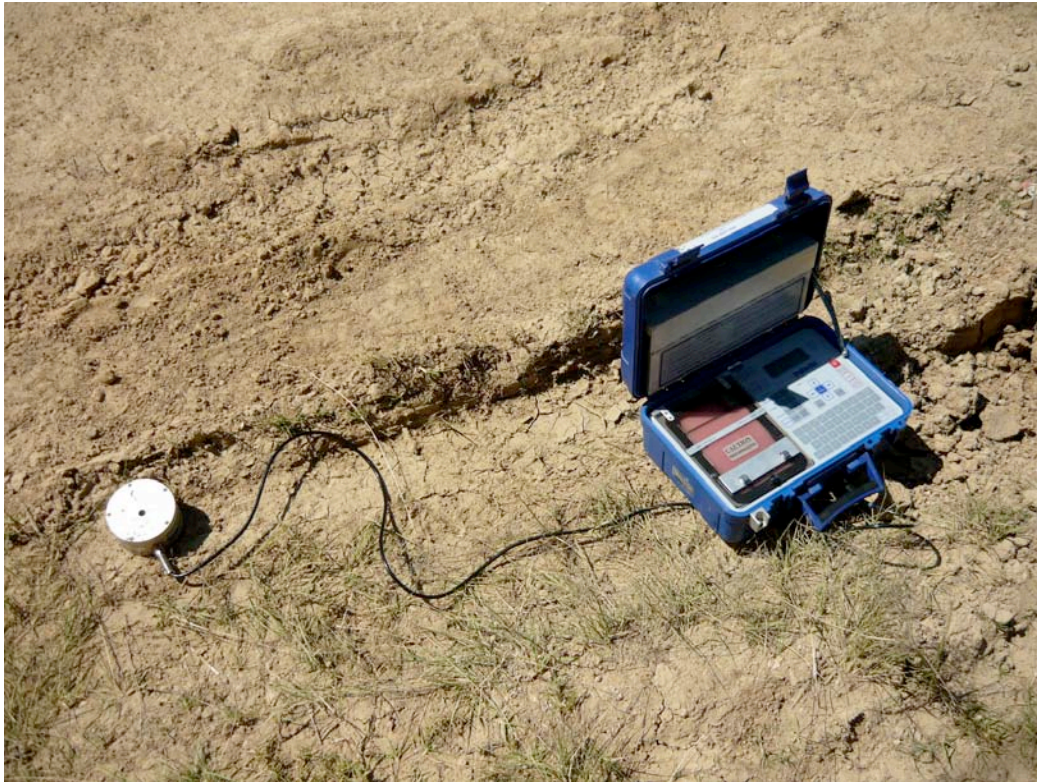
Figure 12a Blastmate III (Sensor on Left, Data Recorder on Right)
